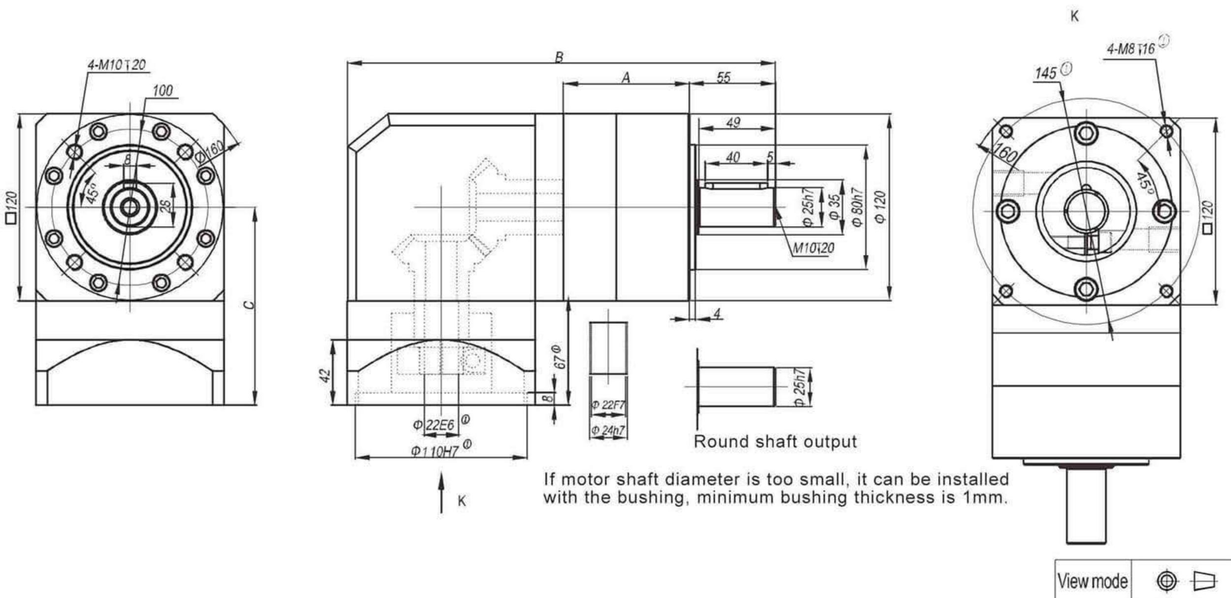
If motor shaft diameter is too small, it can be installed with the bushing, minimum bushing thickness is 1mm.
