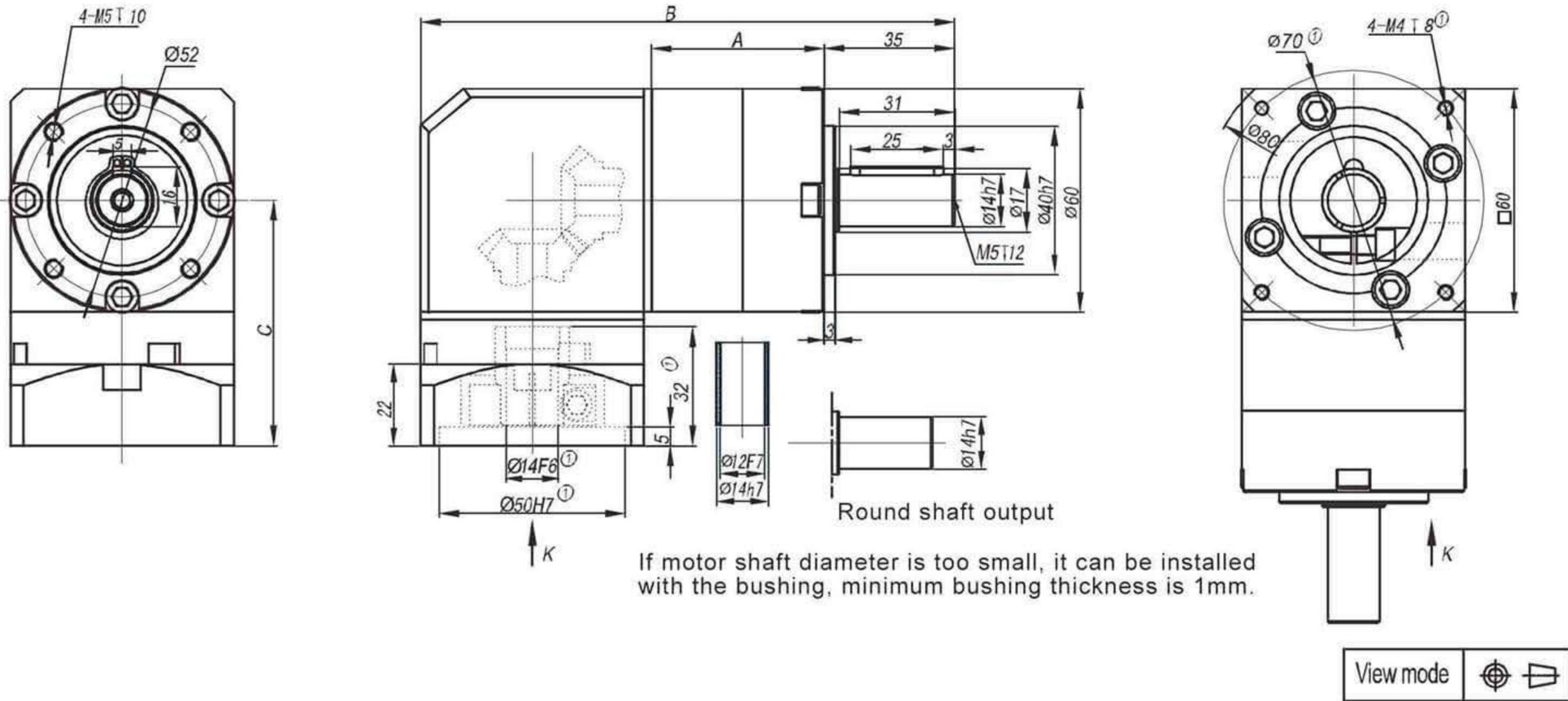
If motor shaft diameter is too small, it can be installed with the bushing, minimum bushing thickness is 1mm.
